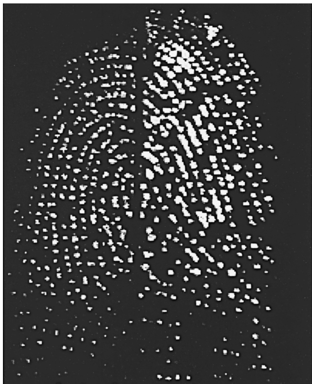
FIG. 13—Comparison of DFO and 1,2-indanedione with zinc treatment in petroleum ether on photocopy paper cooled by liquid nitrogen. Left side: DFO. Right side: 1,2-indanedione with zinc ( \lambda_{ex} 555 nm and \lambda_{em} 610 nm).
